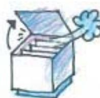
Open the battery cover so that gasses can escape during charging
