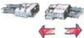
Disconnect the battery connector and the charger connector
